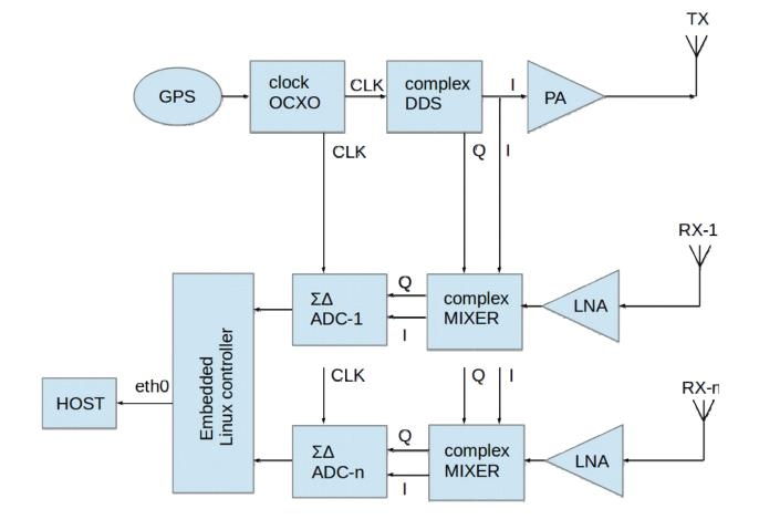
*Principle of operation:* the signal generator is programmed to emit a repetition of ramps (chirp), typically of a duration of 0.2 to 1 s and a bandwidth of 30 to 300 kHz determined by the frequency allocation obtained from the national agencies, resulting in a frequency modulated continuous wave (FMCW mode).
