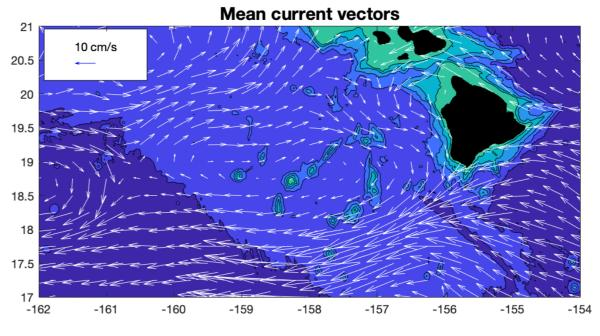
The bathymetry of South Point and associated mean currents.
