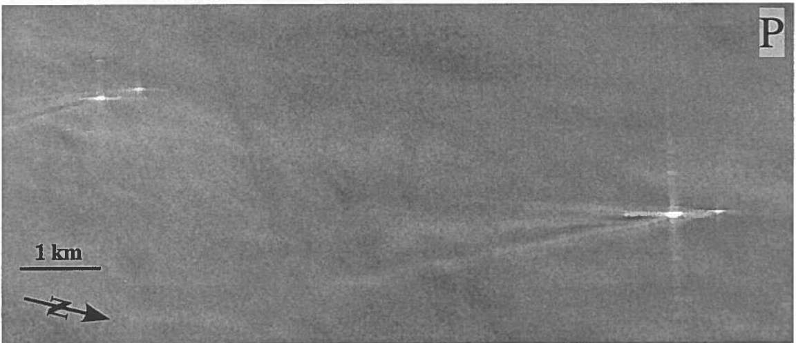
Figure 22. Detail of ships. Ghosts and bars about the ships likely result from the high radar cross-section of the ships combined with beam side-lobe and electronics effects. Bow and stern wakes are visible. The prominent disturbance of surfactants produced by the stern wake is 170 m wide.
