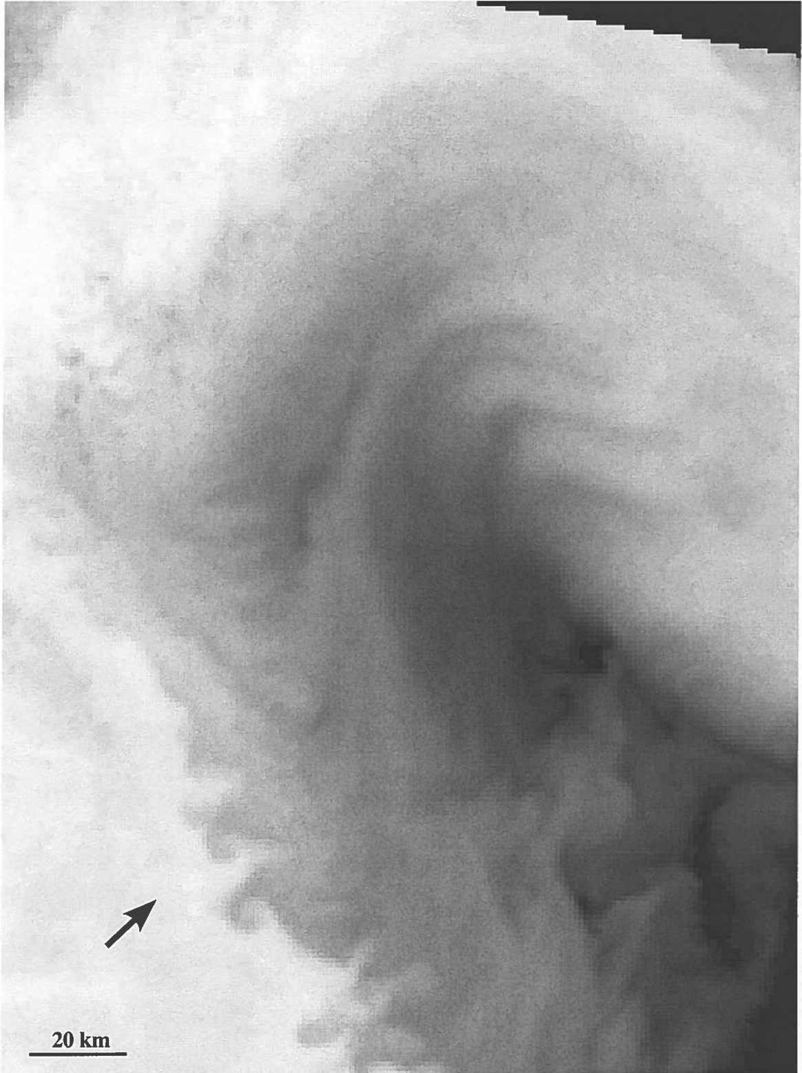
Figure 9. Detail of region A (see figure 3), AVHRR channel 4 at JD 250, GMT 13:36. The apparent instability train indicated by the arrow is moving SSE at \sim 0.2 m/s.
