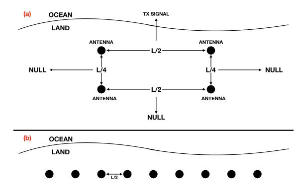
Figure 5.2: (a) Transmit antenna array showing distances between antennas, cable delays, and orientation with respect to the ocean to create three directional-nulls and amplify the signal over the ocean. (b) Receive antennas array for HFRs with spacing less than half the radio wavelength (L). Array is oriented parallel to coastline.
