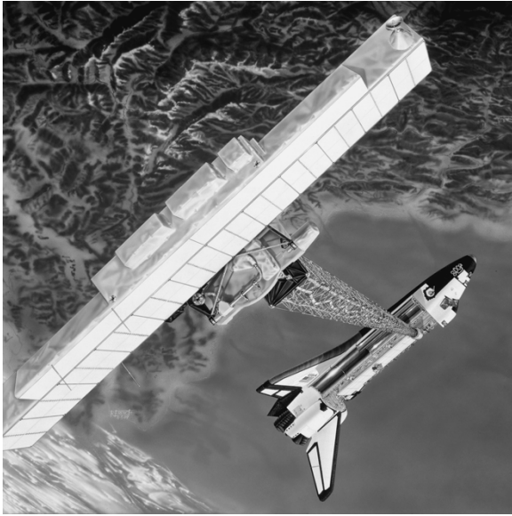
Fig. 1. Artist's view of the SRTM configuration in space. Note that the mast with the outboard antennas is installed ahead of the main antennas in the cargo bay, which leads to an along-track separation of 7 m between the phase centers of the main antennas and the outboard antennas. Courtesy of Ball Aerospace & Technologies Corp.
