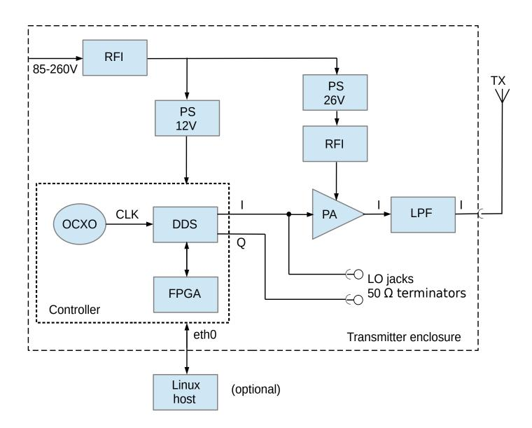
*Figure 1. Schematics of the Synthesizer-Transmitter Unit. See Table 2 for list of components and references.*
