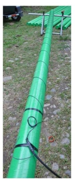
Figure 6. Normal-mode helical monopole with air-coil on a fiberglass mast (8 MHz).
