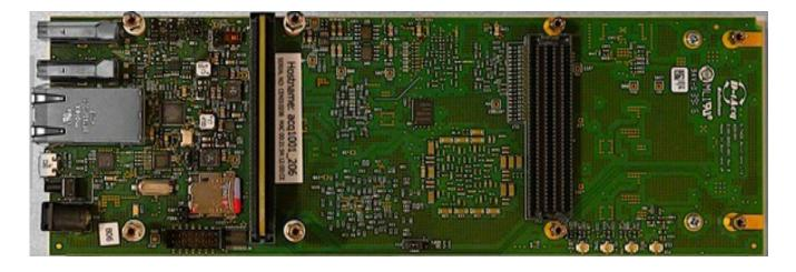
Figure 3c. Photo of the carrier board with FPGA (top face; bottom face not accessible).
