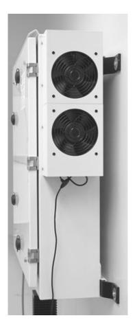
Figure 5. Synthesizer-Transmitter Unit, right side view. The twin-fan forced air flow heat exchanger unit is seen.
