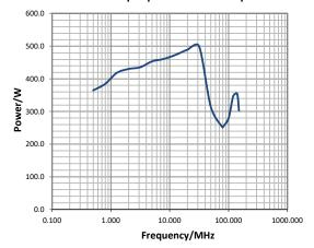
RF input for 50W CW out at +28V DC
