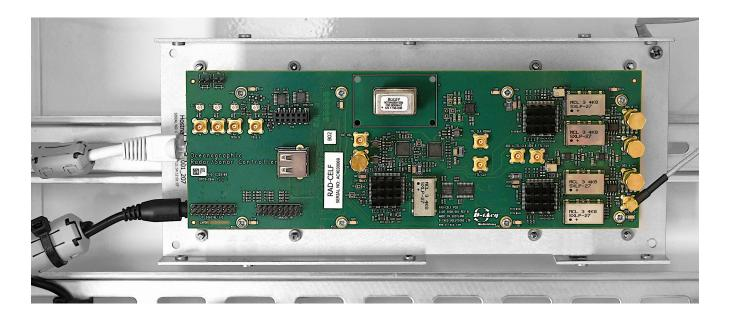
*Figure 11. Upper rail enlarged from Figure 9 and 10, after removal of the aluminum lid and thermal bell, showing the Triple DDS Radar Controller board.*
