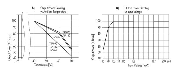
All specifications valid at nominal input voltage, full load and +25°C after warm-up time unless otherwise stated.
