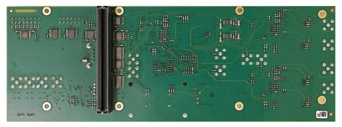
Figure 3b. Photo of the Triple DDS Radar Controller board (bottom face).
