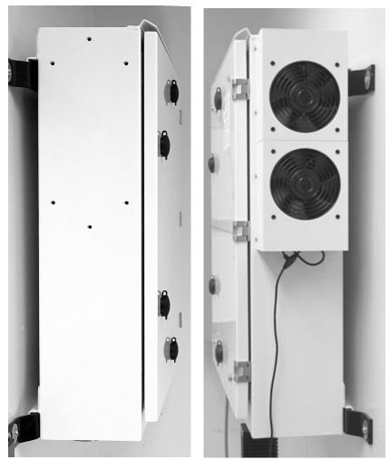
*Figure 2. Synthesizer-Transmitter Unit, left and right side views. The twin-fan forced air flow heat exchanger unit is seen on the right side.*
