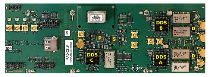
Figure 3a. Photo of the Triple DDS Radar Controller board (top face).
