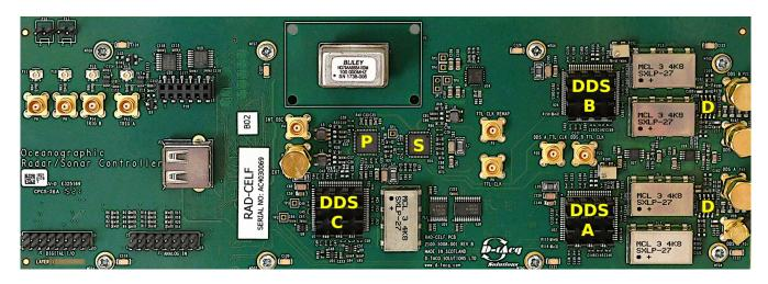
Figure 3. Photo of the Triple DDS Radar Controller board.
