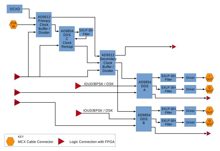
*Figure 2. Schematics of the Triple DDS Radar Controller. See Table 2 for list of components and references.*
