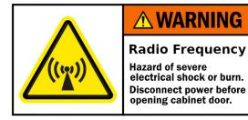
This device contains potentially dangerous high voltages and high frequency radiation. Operation and servicing is restricted to properly trained and certified personnel.
