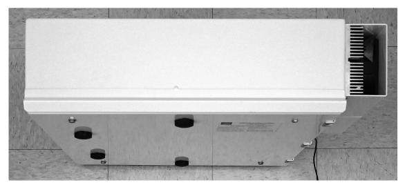
Fig. 4. Synthesizer-Transmitter Unit, top view. The twin-fan forced air flow heat exchanger unit is seen on the right side.
