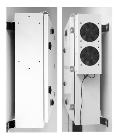
*Figure 13. Synthesizer-Transmitter Unit, left and right side views. The twin-fan forced air flow heat exchanger unit is seen on the right side.*
